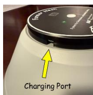
Figure 2 Location of Charging Port on FN Animal and Insertion Orientation of Charging plug
